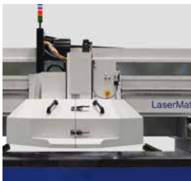
The laser on-board protection hood together with the light barriers allow direct crane loading as well as loading and unloading during the cutting operation
