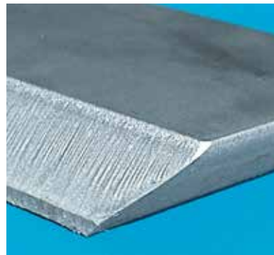
Bevel example in Mild Steel: 15 mm 45° YDS and 30° VAS (cut quality depends upon material)
